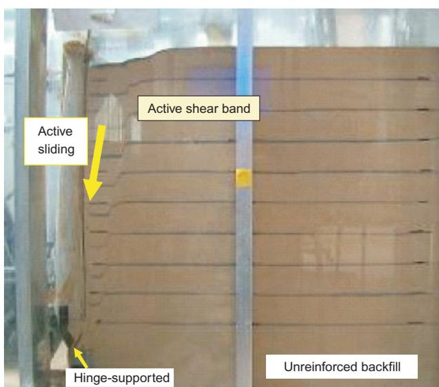
**Figure 13.** Typical active failure in unreinforced backfill developed by lateral cyclic displacement of facing;  $D/H = 0.2\%$  (active only)
